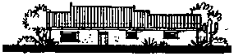
Not Acceptable: Ridgeline too undifferentiated.
